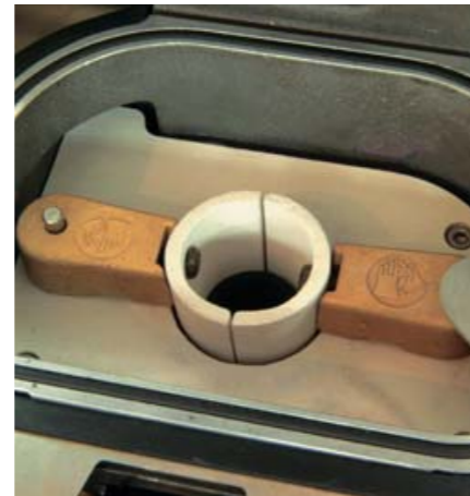
Lifting crucible with inserted graphite ingot to reduce oxygen during gold casting
