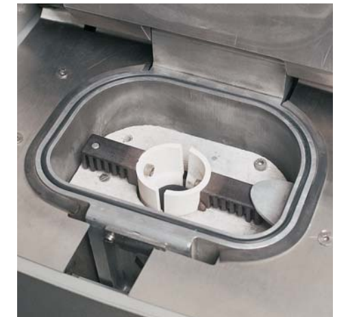
Lifting crucible with inserted graphite cylinder for the oxygen reduction during gold casting
